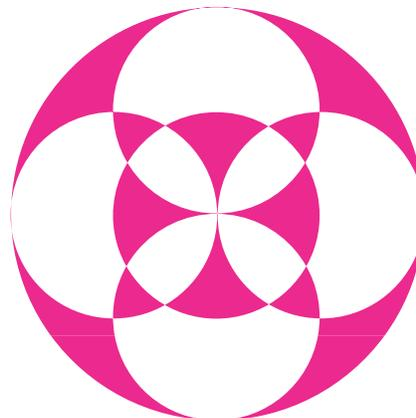
Fig 5. The Ambisonic logo indicates the components of a B-Format signal: the outer circle represents the omnidirectional feed, W; the vertical figure-8 front minus back (X); the horizontal figure-8 left minus right; and the center circle is the up minus down (Z) figure-8 seen from above.
