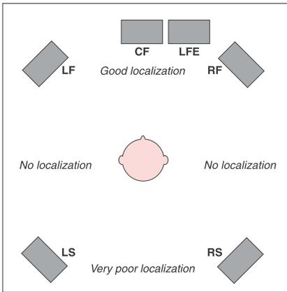
Fig 4. Today's "5.1" systems are based on "discrete quad", with a center-front channel to fill the hole between the front speakers - fine for dialog, but difficult to integrate in music mixing. And the localization everywhere else is as bad as before.
