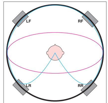
Fig 3. Matrix quad tried to get the four original channels into two and back again, which is impossible. A sound panned around the control room in a circle (black) would be replayed as a flat ellipse by SQ (red) and a cardioid shape (blue) by QS (the foundation for Dolby Surround).
