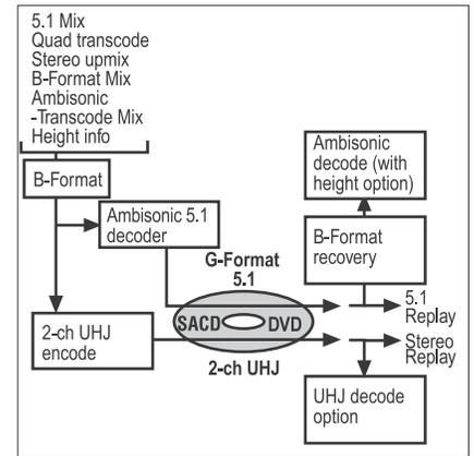
Fig 9. The author’s “G+2” proposal includes Ambisonic information pre-decoded for 5.1 (“G-Format”), for direct surround replay, yet providing for B-Format recovery, plus a 2-channel UHJ mix that can be replayed by any player and decoded for surround if desired.
