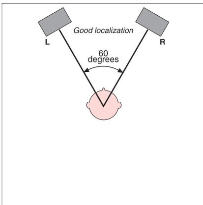
Fig 1. "Intensity" or "amplitude" stereo relies on level only to localize sounds between the speakers. If the ears hear both speakers (ie they are at 60 degrees or less) and at the front, we convert the amplitude differences into phase differences: it works.
