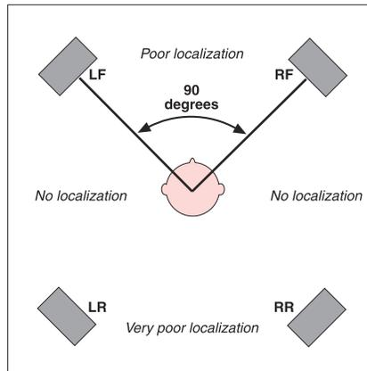
Fig 2. "Quad" relied on speakers at 90 degrees, around the listener. The spacing is too great and sounds are drawn into the speakers: localization is poor at the front, very poor at the rear and nonexistent elsewhere.
